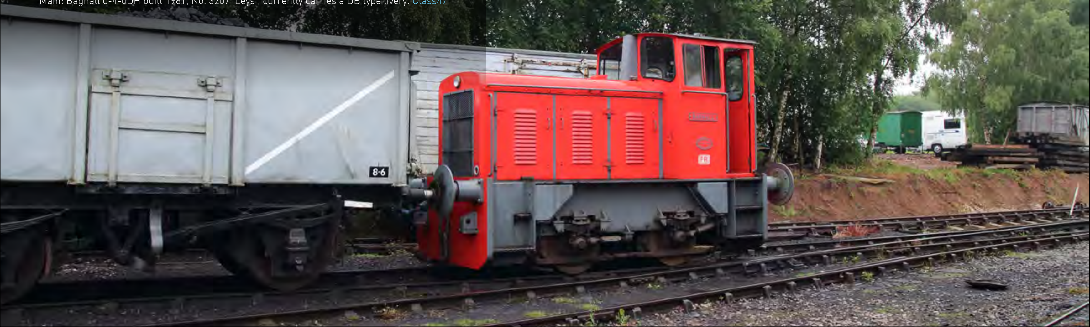
Main: Bagnall 0-4-0DH built 1961, No. 3207 'Leys', currently carries a DB type livery. Class47
