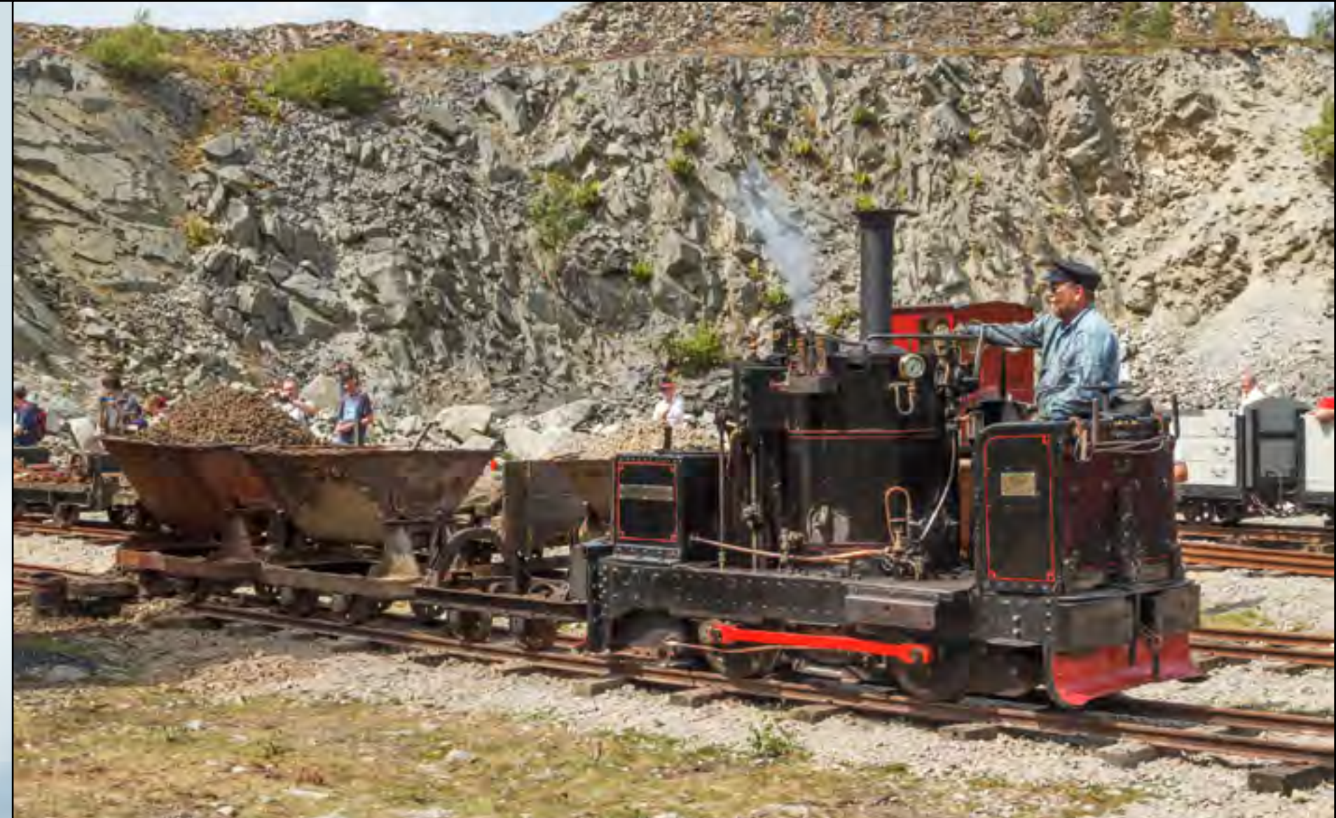
Right: Visiting from Leighton Buzzard Railway, 0-4-0VB 'Chaloner' built in 1877 by De Winton in Caernarfon for use in the North Wales slate quarries, is seen moving loaded tipper wagons of ballast at the back of the quarry. Ken Abram
