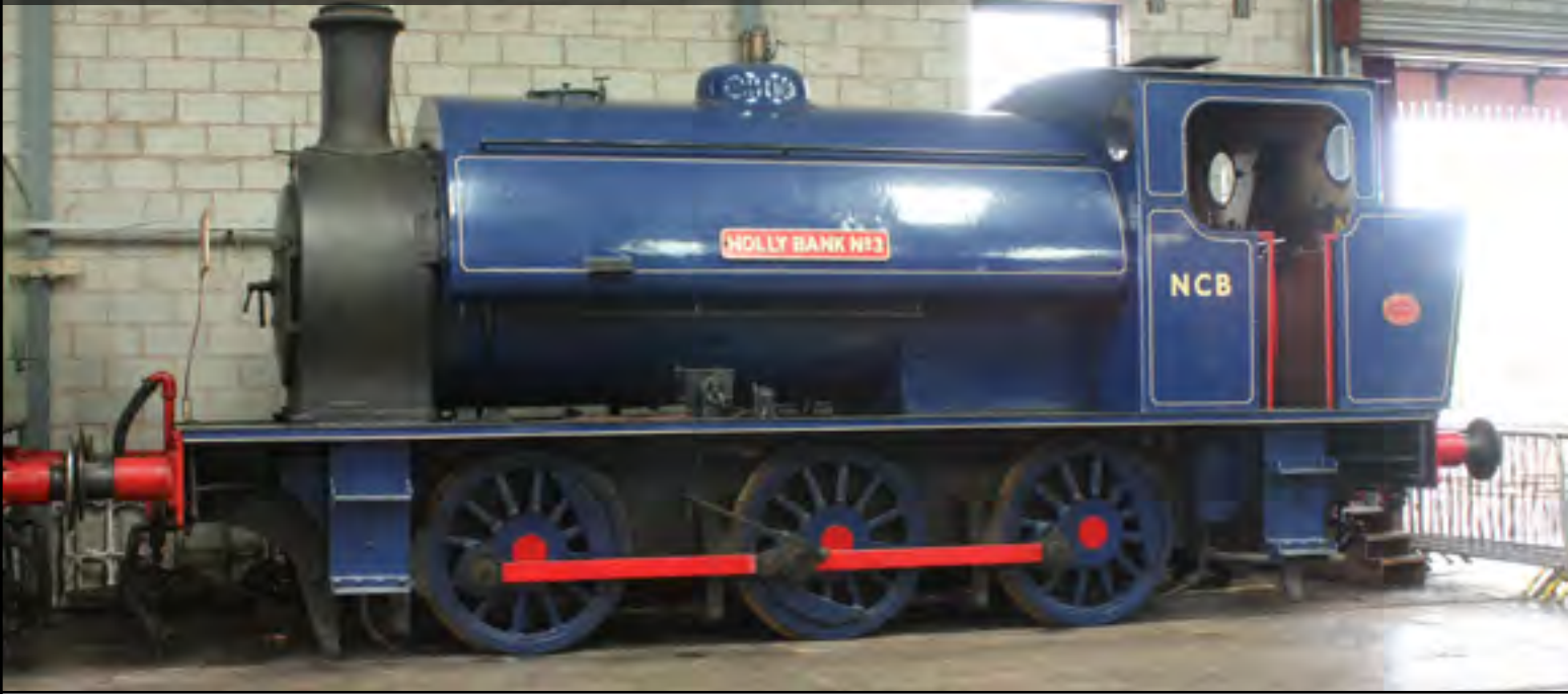
Above: Hunslet of Leeds 0-6-0ST Hollybank No 3. awaits attention in the shed. Derek Elston
