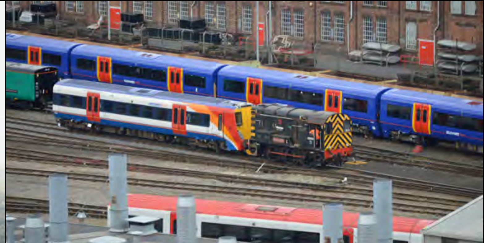
Above: The DMSO of South West Trains Class 458 004 is shunted about Wabtec by 08 669, on it's way to being converted to a Class 458/5. Alex Thorkildsen
