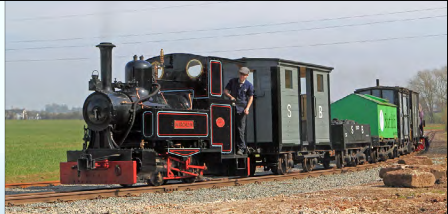
Above: Marchlyn 0-4-0ST from Avonside Engineering works No. 2067 of 1933 is seen returning the freight train to Statfold. Ken Abram
