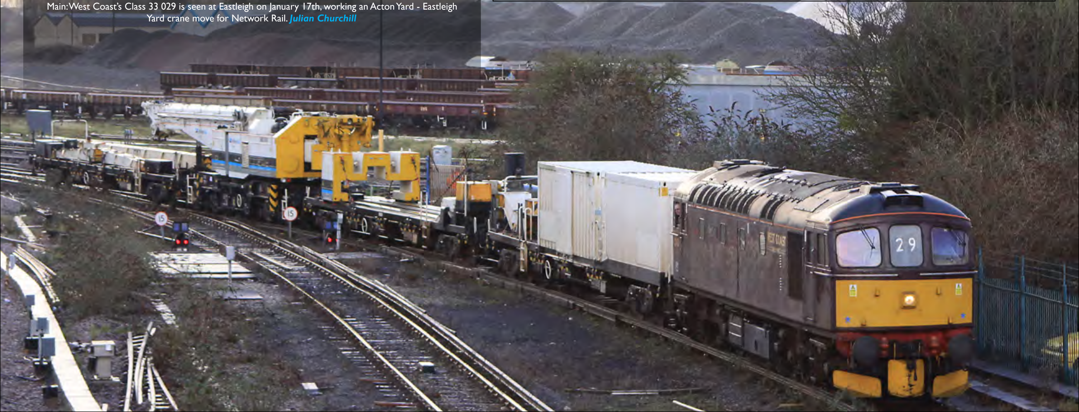
Right: With DBSO No. 9701 leading, Class 37 682 is seen pushing the IQ28 Longsight to Longsight test train through Ashton Moss on January 15th. Brian Hewertson
