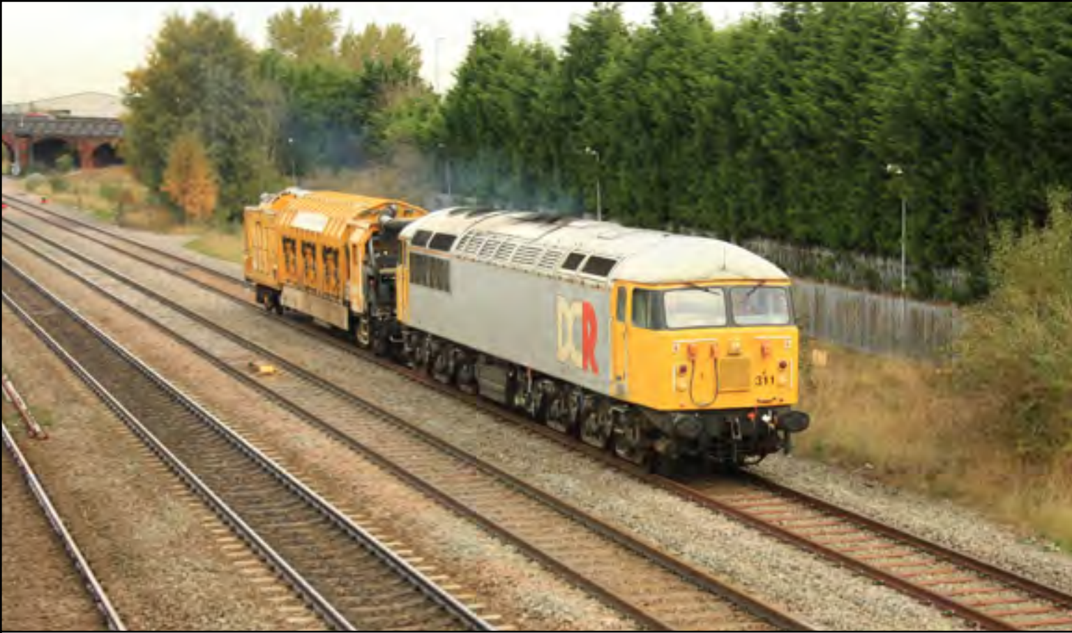
Above: Class 56 311 with the Swedish Railvac machine working 6Z00 Derby Chaddesden sidings to Southampton Totton Yard passes through Burton on Trent, November 9th. Stuart Hillis
