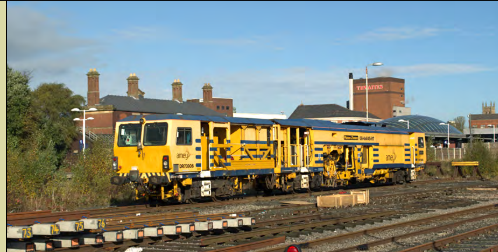
Above: Amey's Plasser & Theurer 08-4x4/4S-RT Switch & Crossing Tamper No. DR73906 'Panther' is seen stabled in sidings adjacent to Blackburn Station November 13th. Dave Felton
