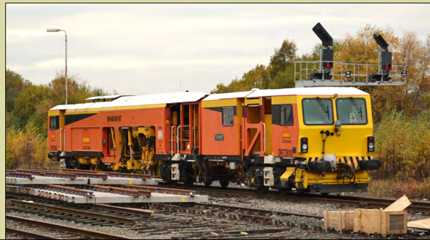
Below: Colas Rail's Plasser & Theurer 08-4x4/4S-RT Switch & Crossing Tamper No. DR73910 'Jupiter' pictured stabled in sidings adjacent to Blackburn Station on November 13th. Dave Felton
