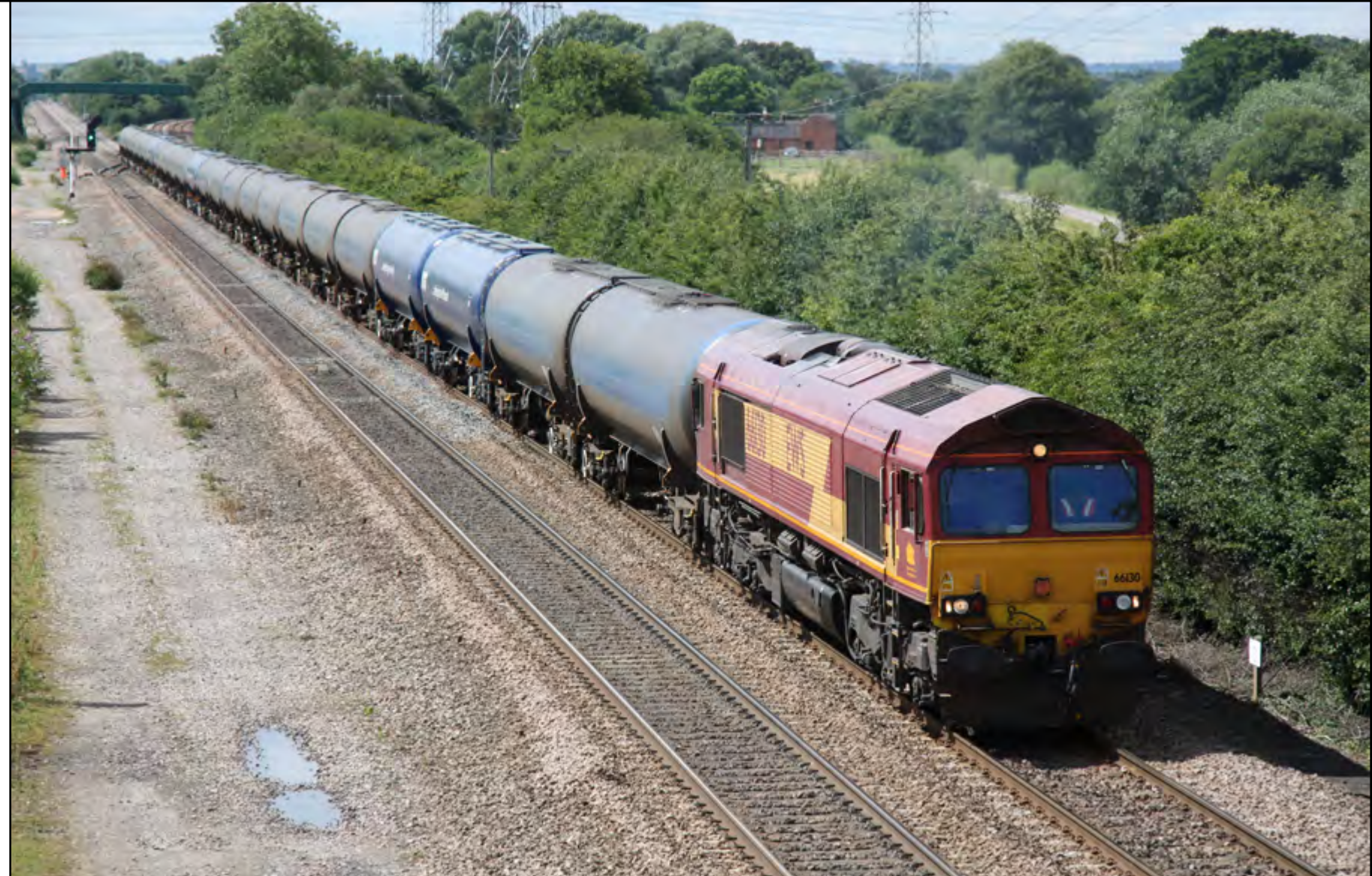
Top Right: Class 66 130 passes Stenson Jct. on July 29th with the Kingsbury - Humber oil tanks. Normally a solid Class 60 turn with 30 loaded tanks, however the Class 66 can only manage 24. Phil Martin
