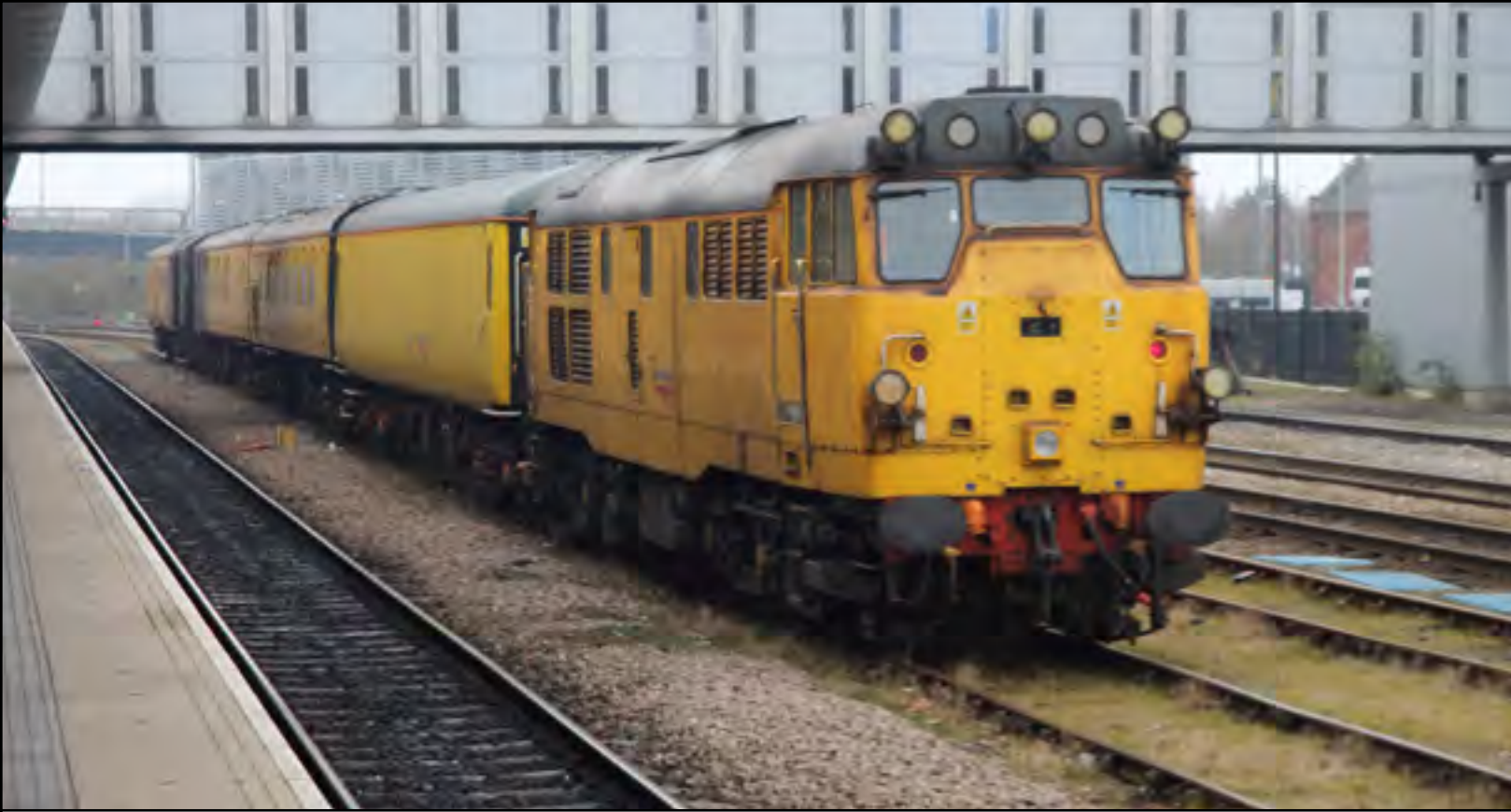
Above: Network Rail's Class 31 233 is seen stabled at Derby station with the tunnel gauging train on March 9th. Class47
