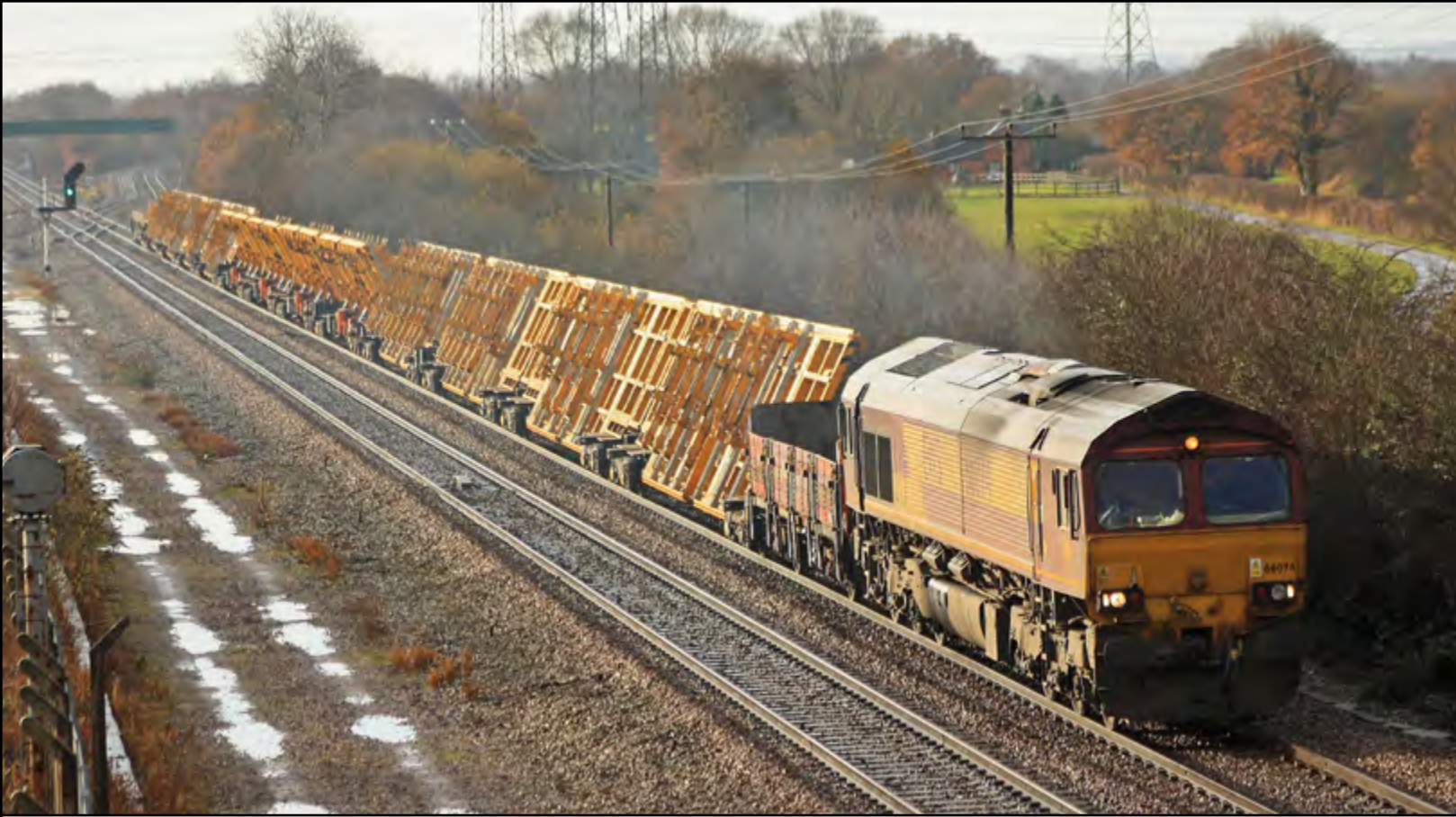
Above: A filthy Class 66 074 working 6D44 Bescot - Toton engineers with a train of point carriers is seen passing over North Staffs Jct. and is about to turn off the main line at Stenson Jct., December 4th. Stuart Hillis
