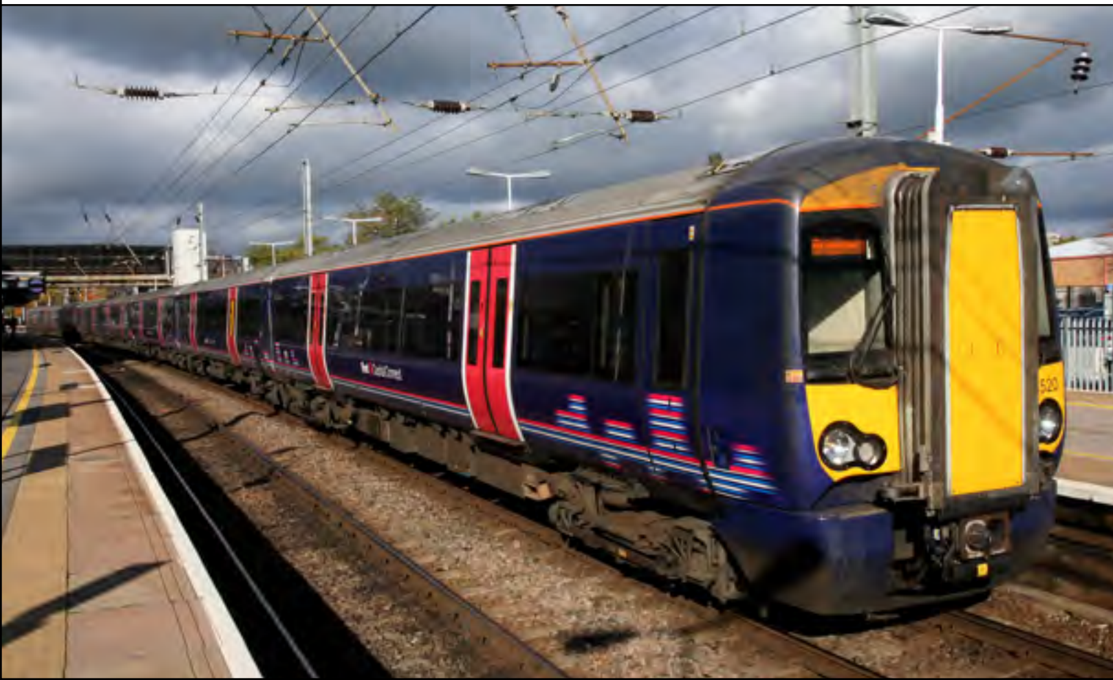
Below: FCC Class 377 520 stands at Bedford station on October 29th. These units now have yellow stripes to identify the disabled passenger doors (just visible on third set of doors). John Coleman
