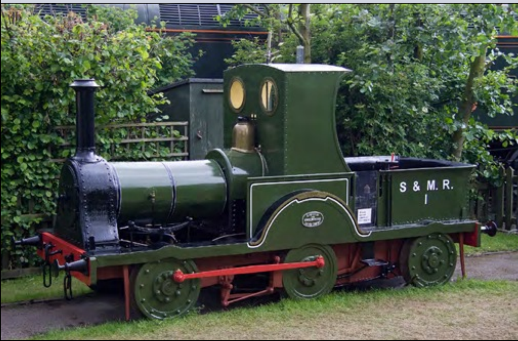
Bottom Left: Probably the smallest standard gauge steam loco in the world, No. 1 "Gazelle", built in 1893 by Alfred Dodman, King's Lynn as a 2-2-2WT for William Burkett. Richard Hargreaves
