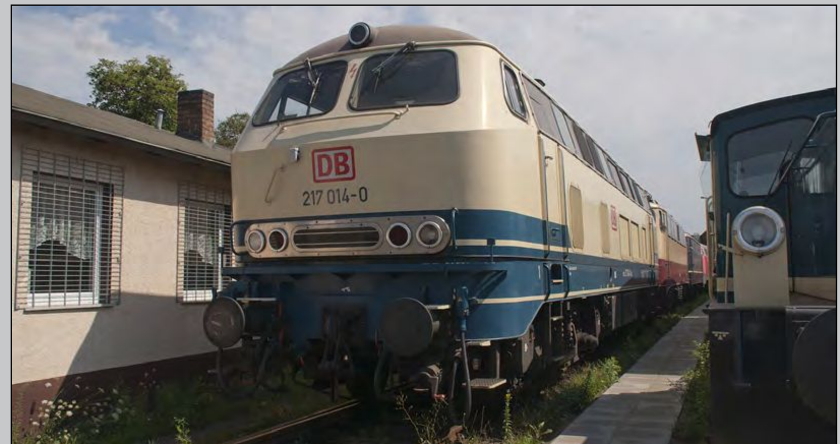
Top Left: Locomotives of the Series E41 were designed to carry light freight and passenger trains. Bottom Left: Deutsche Reichsbahn procured Series E44 locomotives as a universal locomotive for passenger and freight. Top Right: Class 181s were bought by the German Federal Railways for cross-border traffic with Luxembourg and France. Bottom Right: The Class 217 (until 1968 known as Class V162) were bought between 1965 and 1968 and still used today.
