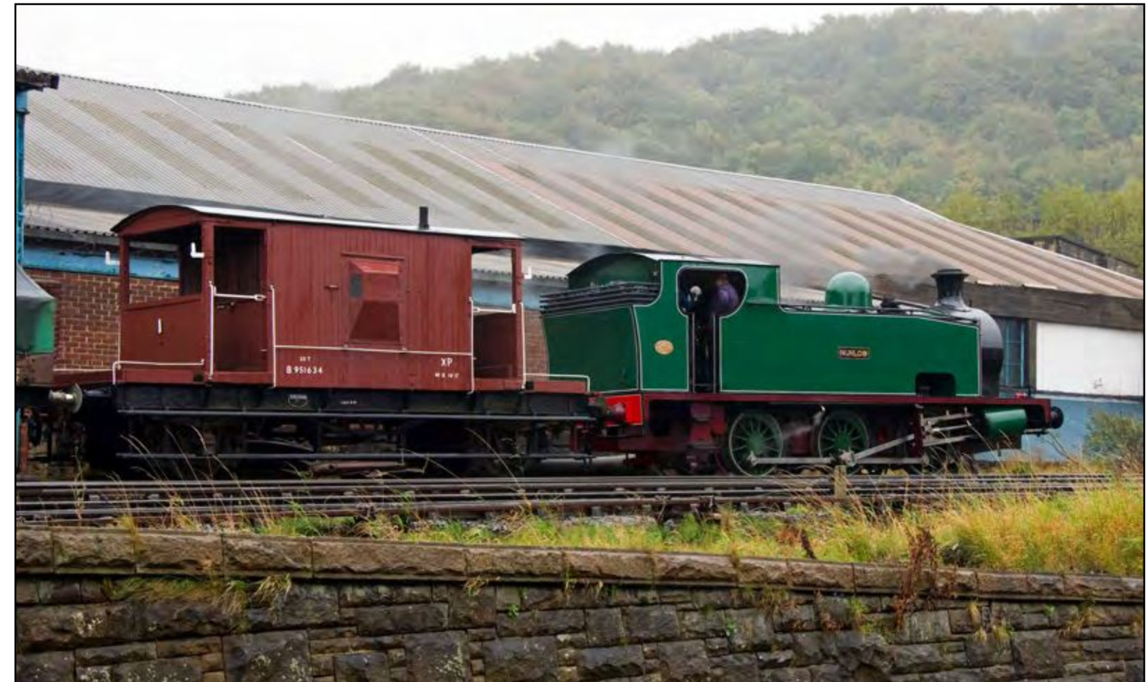
Above: On October 9th, 0-6-0 side tank engine "Nunlow" stands at Keighley with a freight working. This loco was built local to here by Hudswell Clarke & Co Ltd in Leeds. Colin Irwin Below: LMS Black Five 5MT 4-6-0 No. 45212 is seen at Oxenhope on October 7th. Colin Irwin
