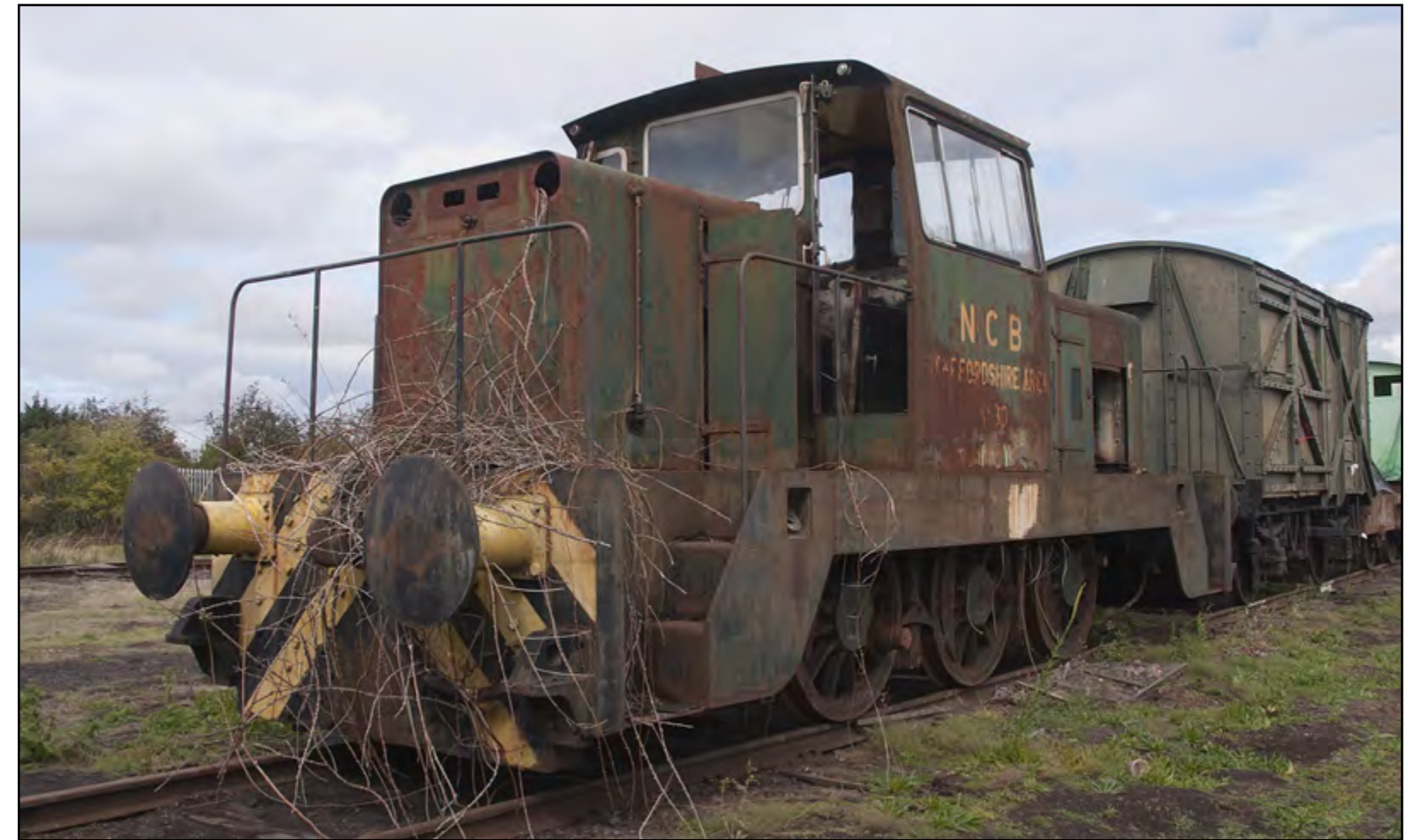
Above: Hunslet Engine Co No. 7181 (NCB No. 30) looks like it has had a fight with a tree, or perhaps a large bird is building a nest. Brian Battersby Below: Hunslet 0-6-0 Diesel Hydraulic, 'Rachael', works number 7003 built in 1971. This loco shunted at the MG Rover Plant at Longbridge until closure in 2007. Brian Battersby
