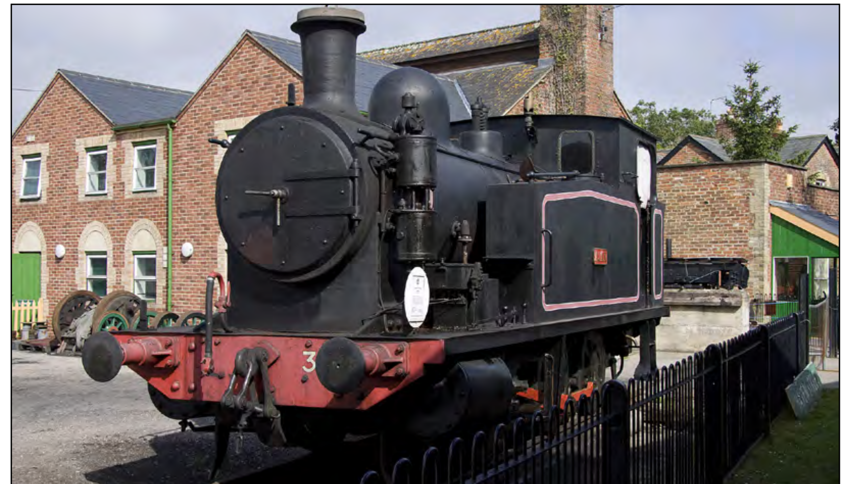
Below: Barclay 0-6-0T No.W38 "Ajax" is seen in the yard at Haven St., Built to the order of the Sulphide Corporation of London in 1918, this loco worked in Persia before returning to the UK. Richard Hargreaves
