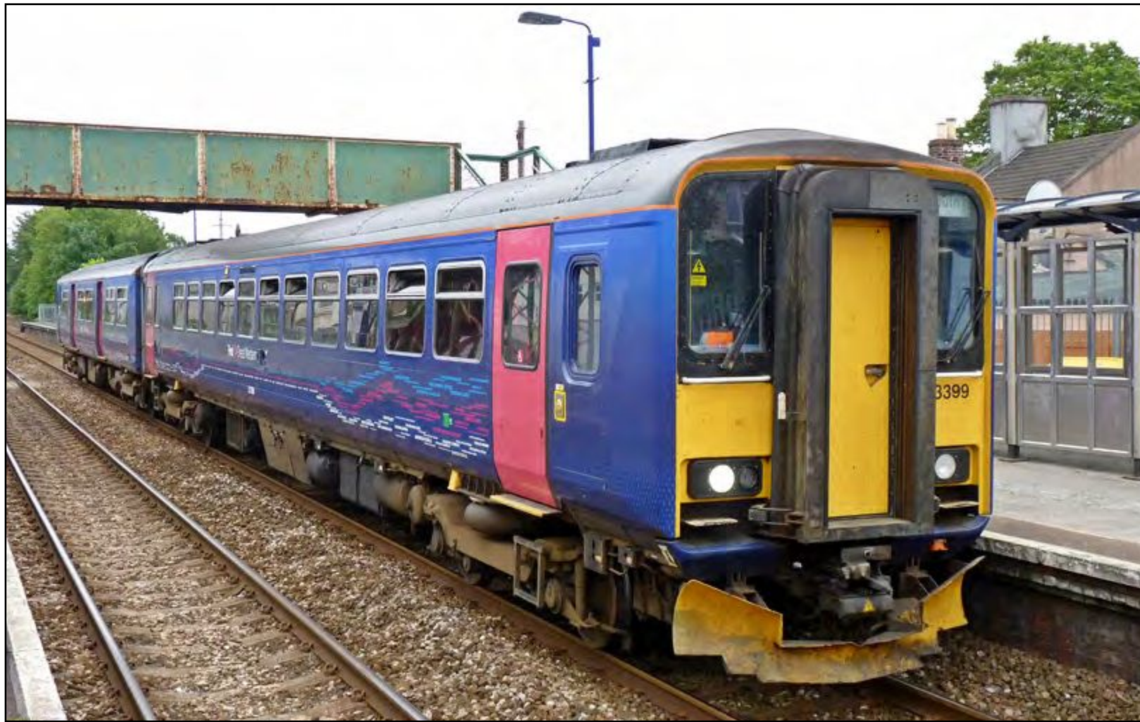
Above: Unique FGW Class 150/153 unit No. 153 399 (Which is 153 369 and half of 150221 (57221)) is seen at Keyham on May 23rd. This pairing is as a result of 52221 sustaining fire damage. Steve Andrews Below: East Midlands Trains Class 153 321 and a Class 158 stand at Stoke on Trent on May 28th with a Derby to Crewe working. Brian Battersby
