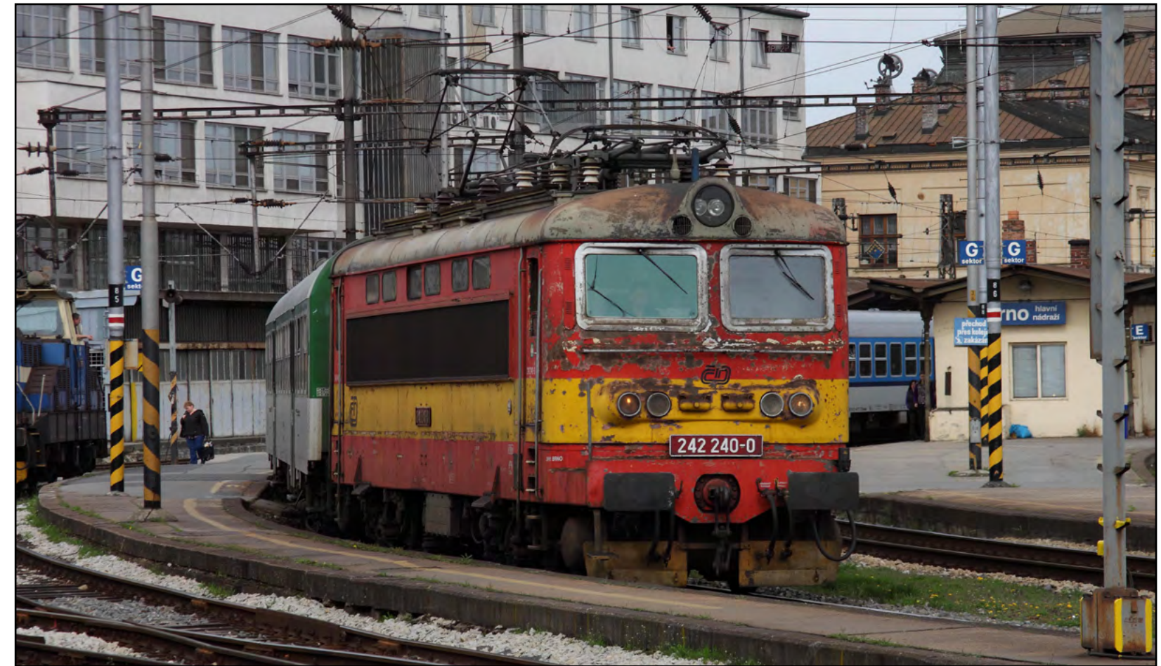
Above: Czech Class 242.240-0, a 25 kV 50 Hz AC electric loco, is seen at Brno Hln having arrived with a stopping service from Tisnov on April 12th. Paul Godding Below: OBB Class 1216.216 speeds through Brno-Zidenice on a drab grey day. Class47
