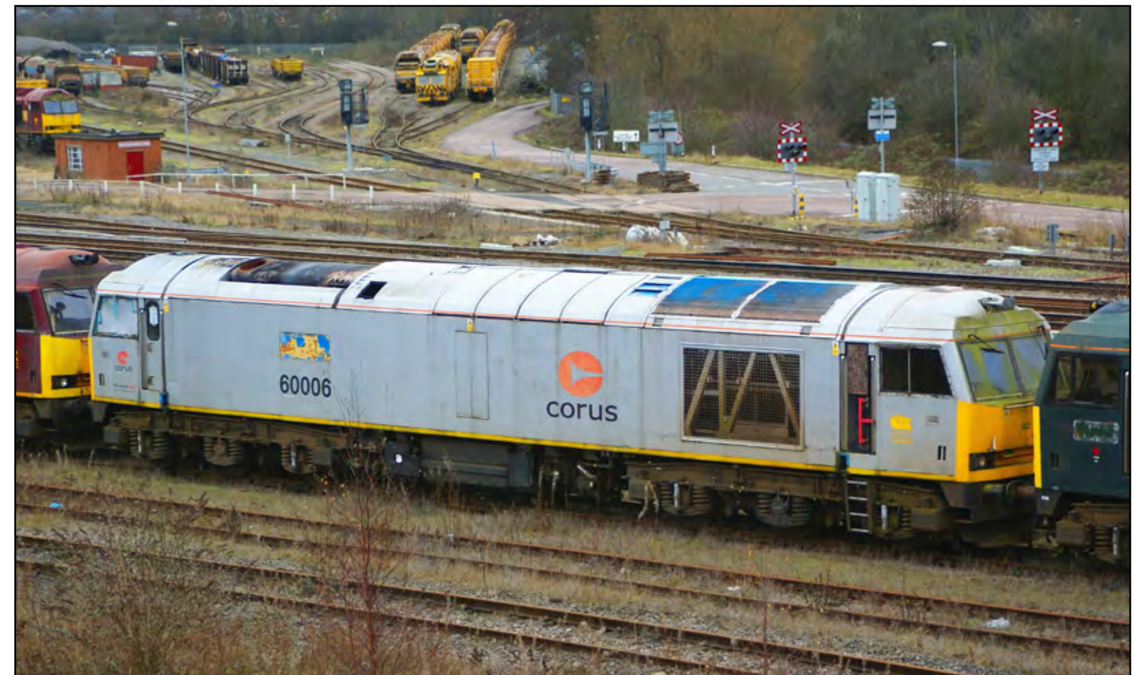
Above: The only green liveried Class 60 081 formally “Isambard Kingdom Brunel” displays the bodyside damage caused as a result of a catastrophic engine failure, occurring near Beeston Castle. This locomotive has been withdrawn since 2005. Dave Harris Below: Corus liveried Class 60 006 formally “Scunthorpe Ironmaster” lies dormant at Toton as a result of fire damage, withdrawn back in 2004. Dave Harris
