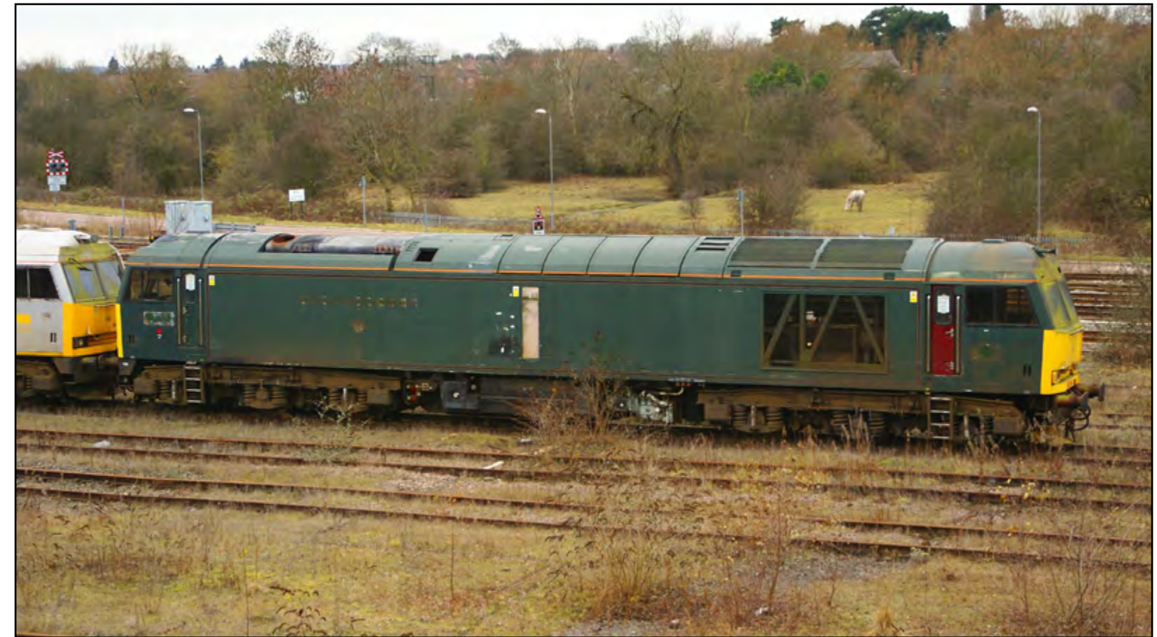
Above: The only green liveried Class 60 081 formally “Isambard Kingdom Brunel” displays the bodyside damage caused as a result of a catastrophic engine failure, occurring near Beeston Castle. This locomotive has been withdrawn since 2005. Dave Harris Below: Corus liveried Class 60 006 formally “Scunthorpe Ironmaster” lies dormant at Toton as a result of fire damage, withdrawn back in 2004. Dave Harris
