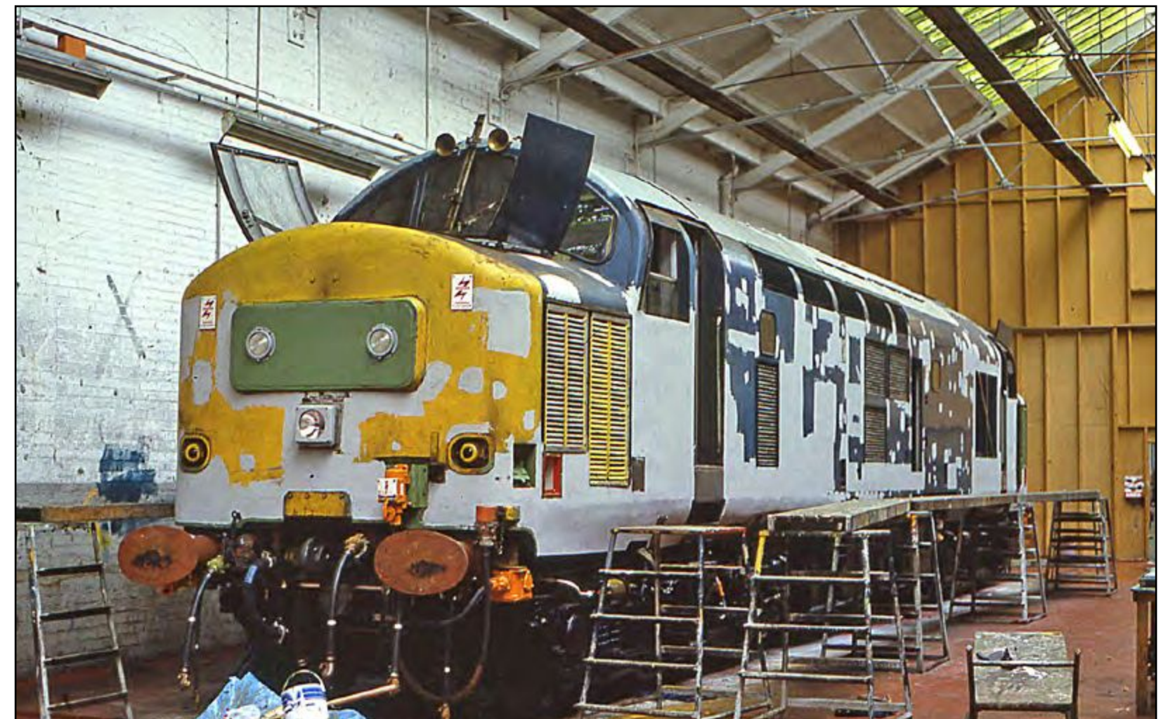
Above: A pair of Class 50s are seen at London Waterloo with services to Exeter in 1982. Derek Elston Below: Class 37 273 gets transformed into 37 410 at Crewe Works on August 11th 1985. Derek Hopkins
