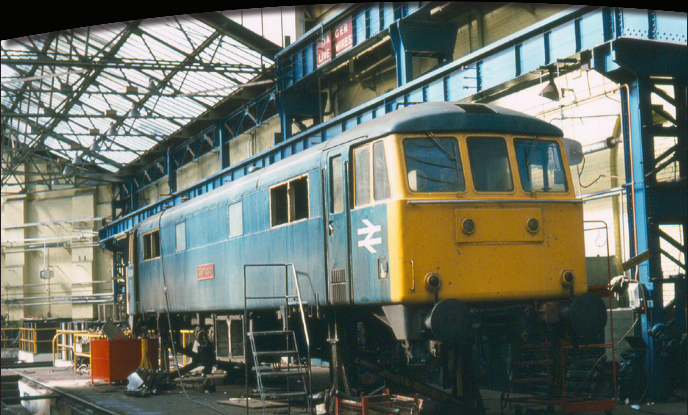
BR AC electric loco Class 86 241 "Glenfiddich" is seen undergoing maintenance inside Crewe Works on April 15th 1984. This locomotive built in 1965 for working the overhead West Coast Main Line was originally numbered E3121 prior to the TOPS system in 1968. The locomotive just survived into the 21st century, being withdrawn early 2000. Crewe Works were had the prime responsibility of maintaining the West Coast fleet, which made sense, as they could be tested easily under the wires. David Mead
