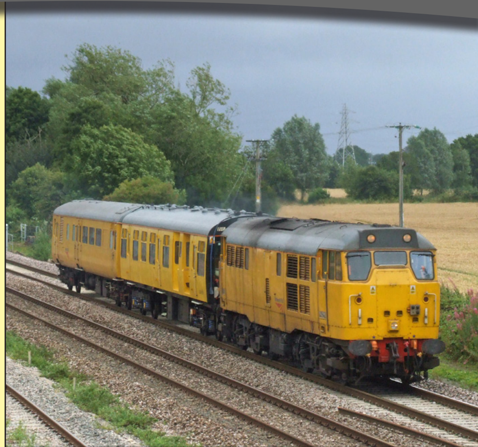
Above: On July 21st, Class 31 285 powers a Network Rail Track Recording train past Norton Fitzwarren whilst working the 2Z08 Westbury to Plymouth Laira. This trip should have been worked by Track Recording DMU no. 95001, but this unit was out of service.
