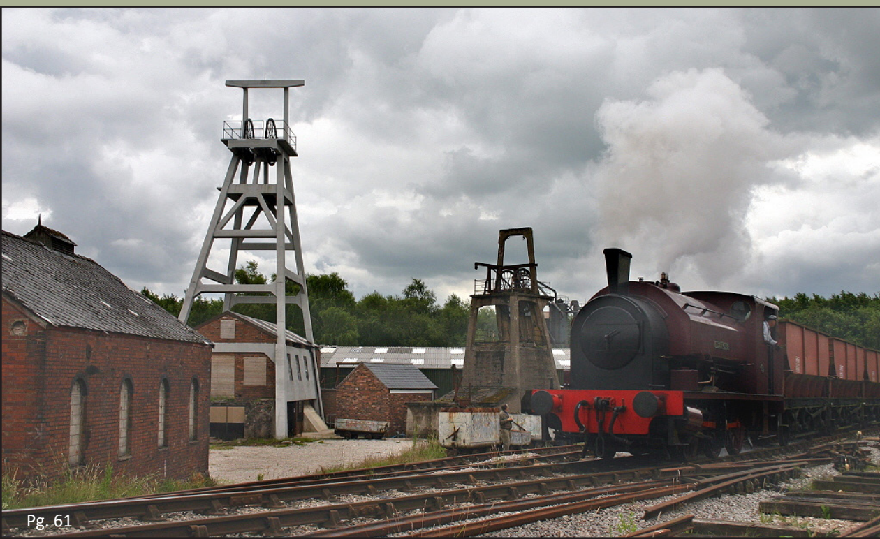
Above: "Meaford No2", a Robert Stephenson and Hawthorn 0-6-0 side tank design, built in 1951 to works number 7684, is seen leaving Foxfield Colliery, as it tackles the, not insignificant, 1:19 climb to Dilhorne. on July 18th. Pete Cheshire
