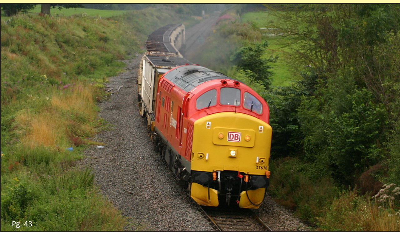
Top Left: Class 97 303 seen in the early hours of July 29th, at Machynlleth. It was undergoing “Odeometer” calibration tests, and wheelslip / wheel skid tests. Extra weight had been placed in the loco, in the form of drums of water, to aid with anti-slip / anti-skid. The wires seen coming from the cab window to the bogie was for measuring wheel-slip. Pete Cheshire
