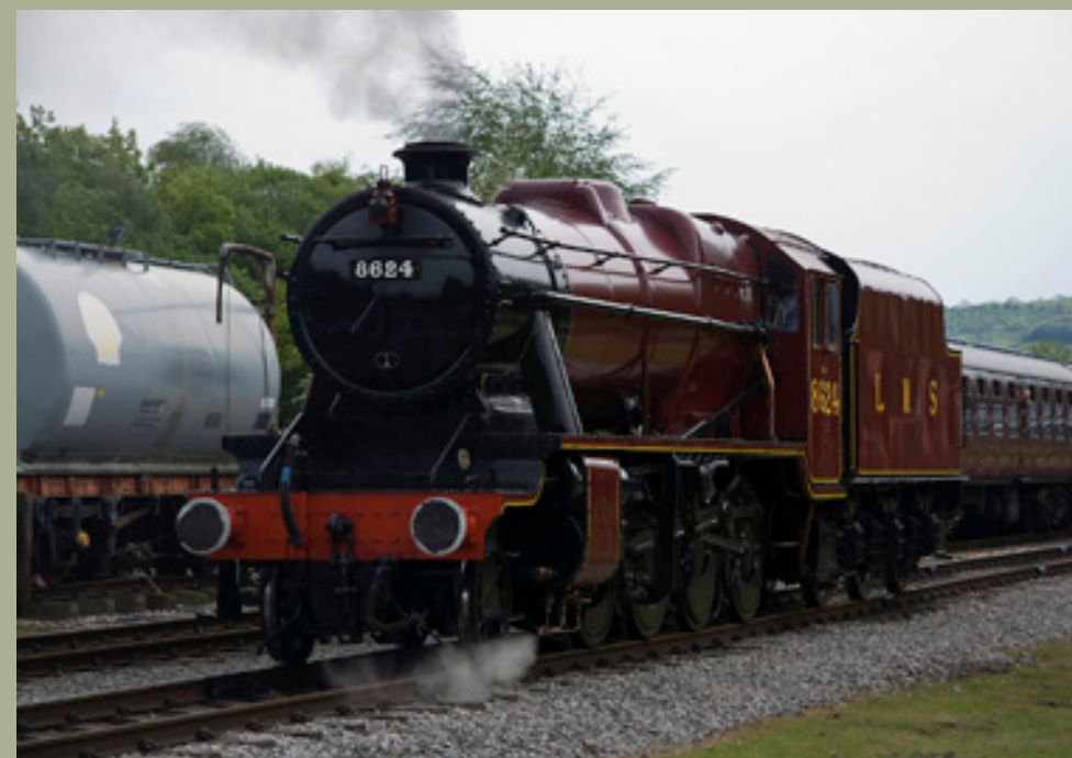
Bottom Right: It has been a long haul for the volunteers from the 48624 Society, but on the weekend of May 25/26th LMS Stanier 8F 2-8-0 locomotive 8624 moved under its own power for the first time in almost 44 years - the end of a 28 year restoration of the locomotive from scrap condition. Richard Hargreaves
