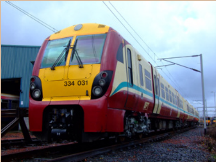
Above: Class 334 031 is seen sitting outside in the yard at Shields T.M.D. awaiting to go through the final tests and exams a C4 overhaul the set received inside the maintenance shed in October. The set was inside the maintenance shed for two weeks in order to complete the C4 overhaul (apart from the tests and exams). A C4 overhaul consists of a set having new bogies, new couplers and a renew of everything underneath the train. Class 334 031 got released from the shed and out into the yard on Friday 31st October and should
