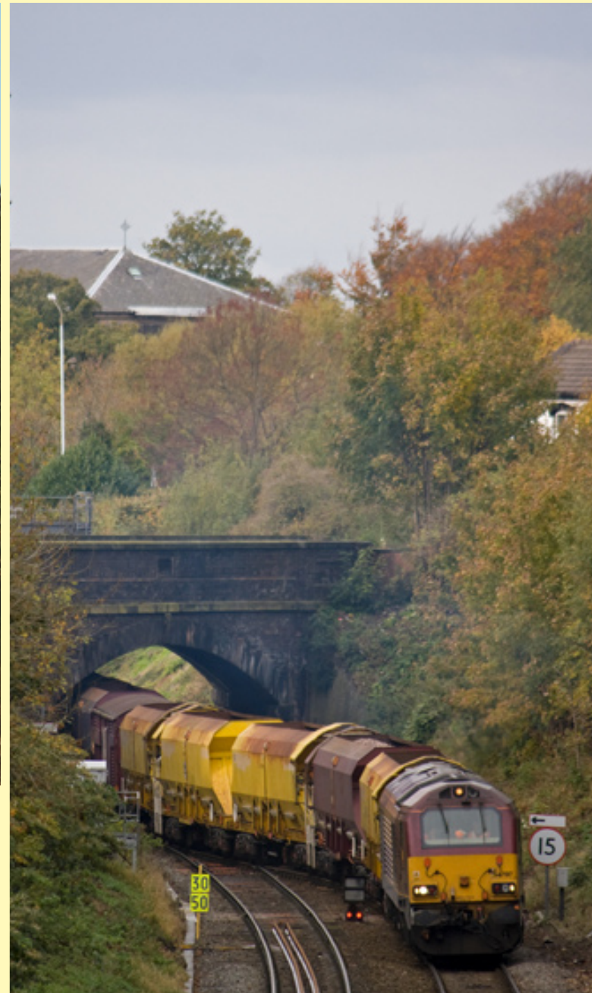
Right: Class 67 017 with 66 105 on the rear, works the 6Z60 Bescot - Wellington Regent Street on the 29th October. The train was dropping ballast on the new Telford Freight Terminal branch as far as Hadley. The terminal is due to open Spring 2009. Carl Grocott
