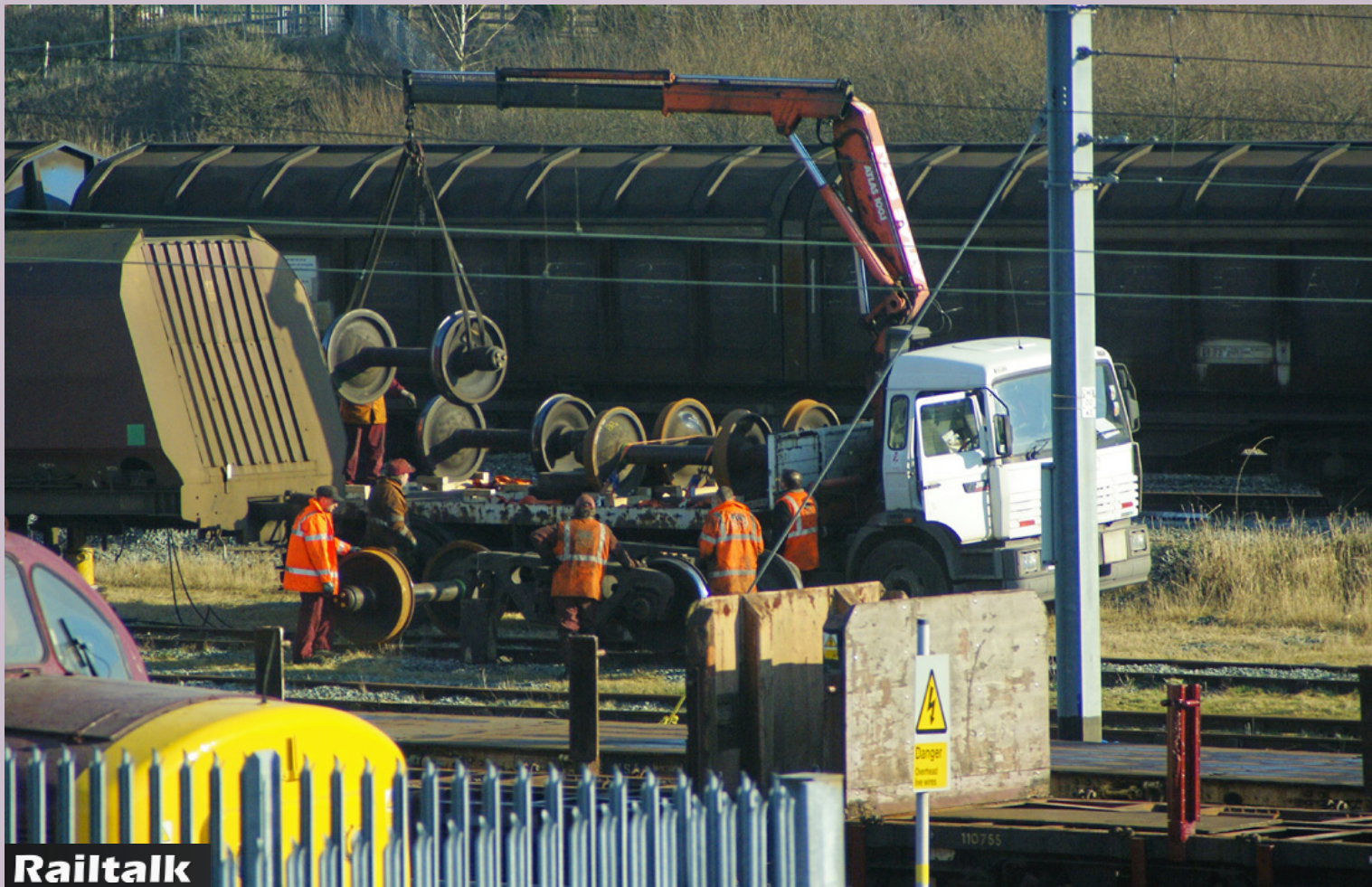
Below: Warrington Arpley on the 16th February, and engineers are trying to replace a set of wheels on a jacked up HHA coal wagon. Dave Harris
