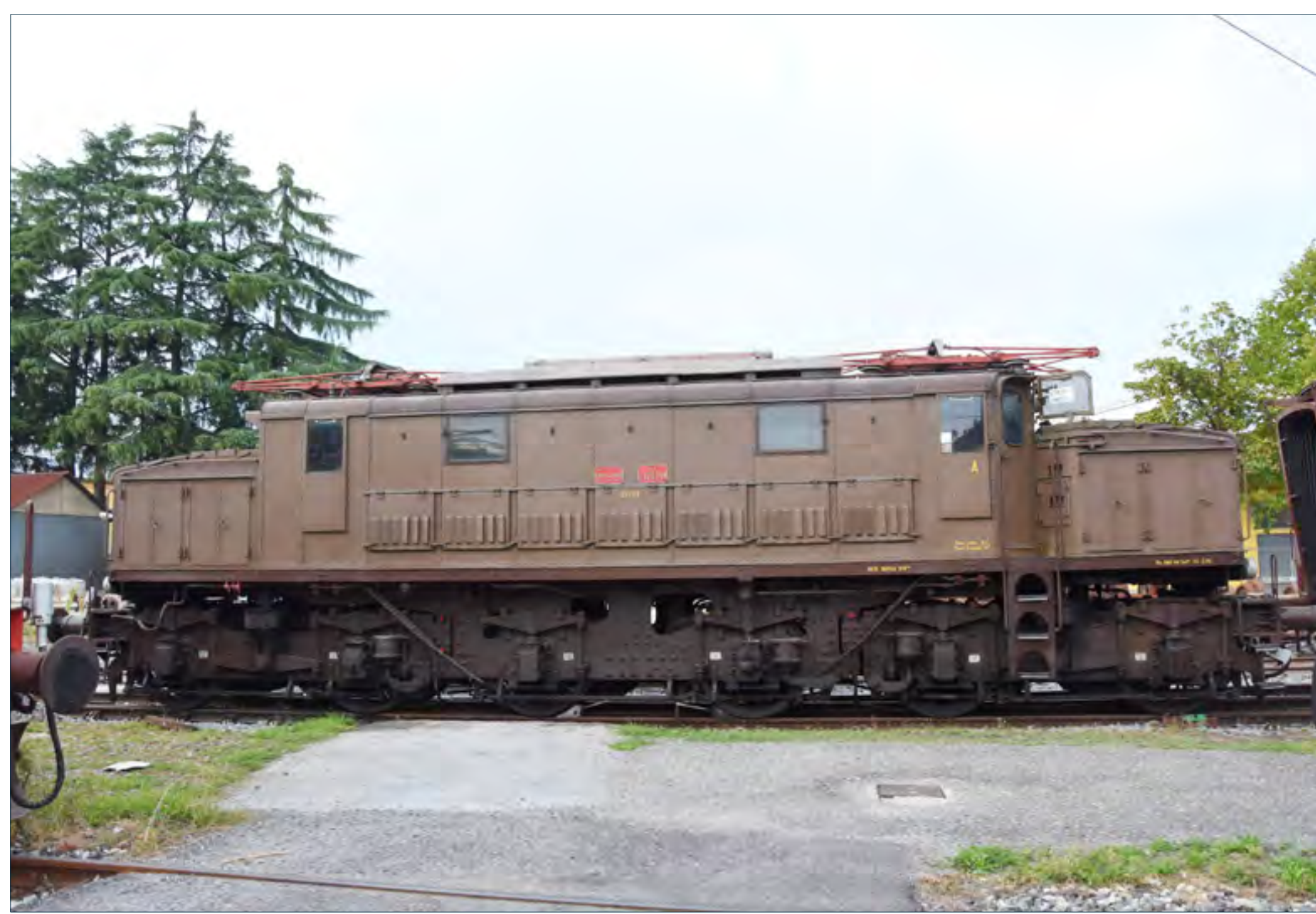
The FS E626 class of Italian electric locomotives were produced for the Ferrovie dello Stato. They were introduced in the course of the 1920s and remained in service until the 1990s, the E626 was the first locomotive fed by 3,000 V DC overhead line in Italy. Preserved No. 626.194 is seen at Pistoia. John Sloane
