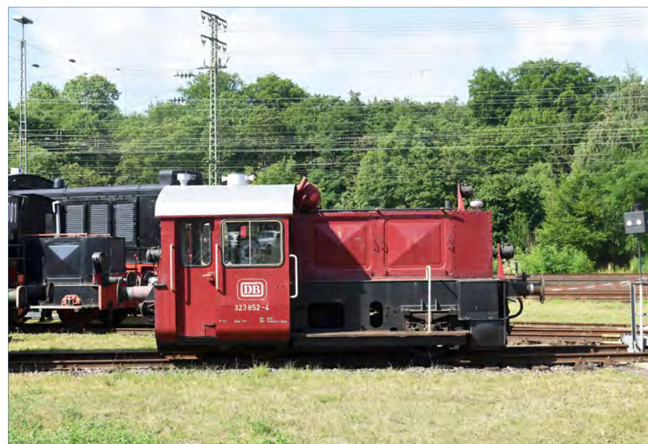
DB shunter Class 323.852 is seen on display at Koblenz-Lutzel museum. This class of locomotives started use from 1932 with the German Reichsbahn and were used at small stations for shunting. John Sloane
