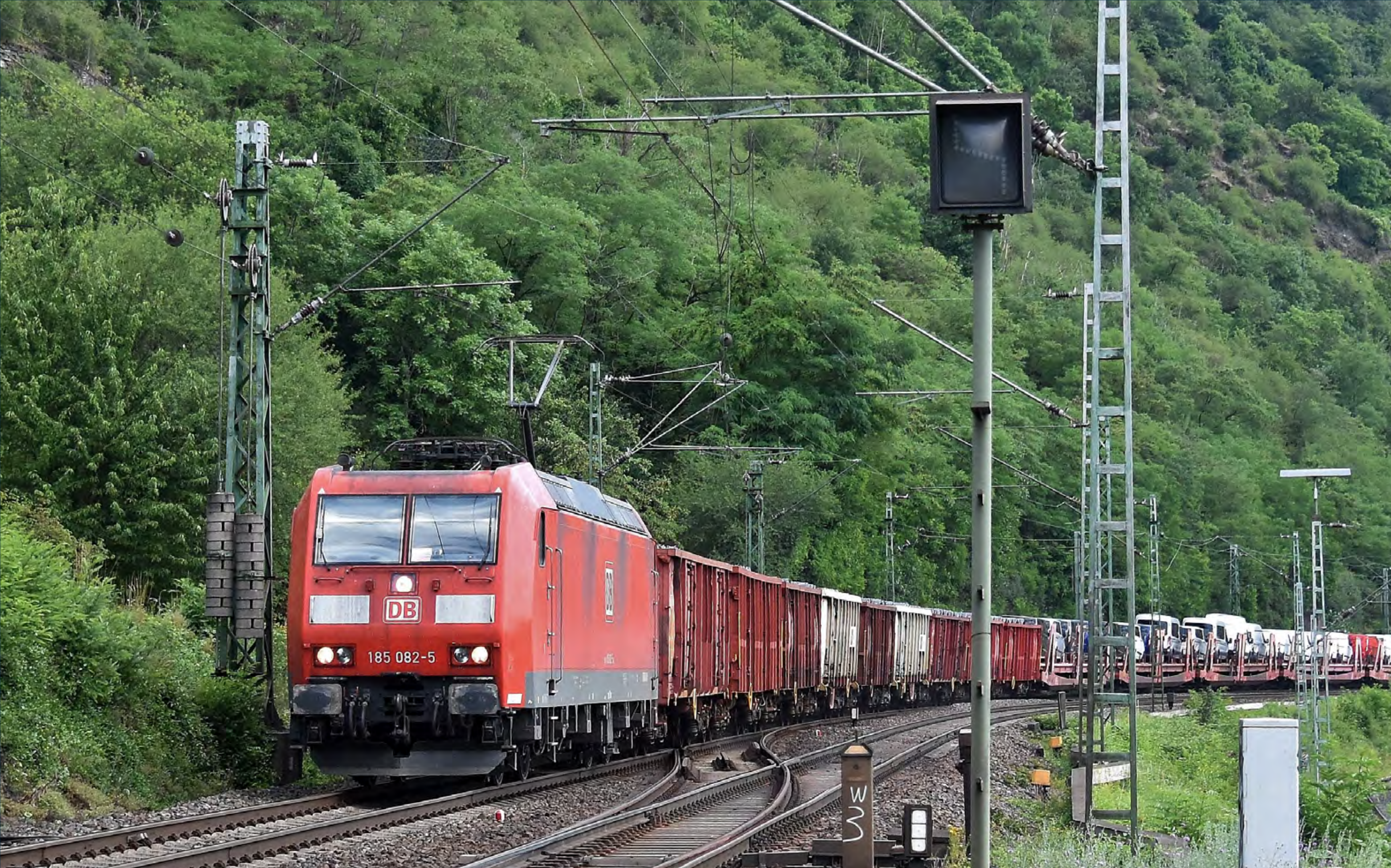
DB Class 185.082 hauls a mixed rake of wagons including some loaded car transporters near Kaub. John Sloane
