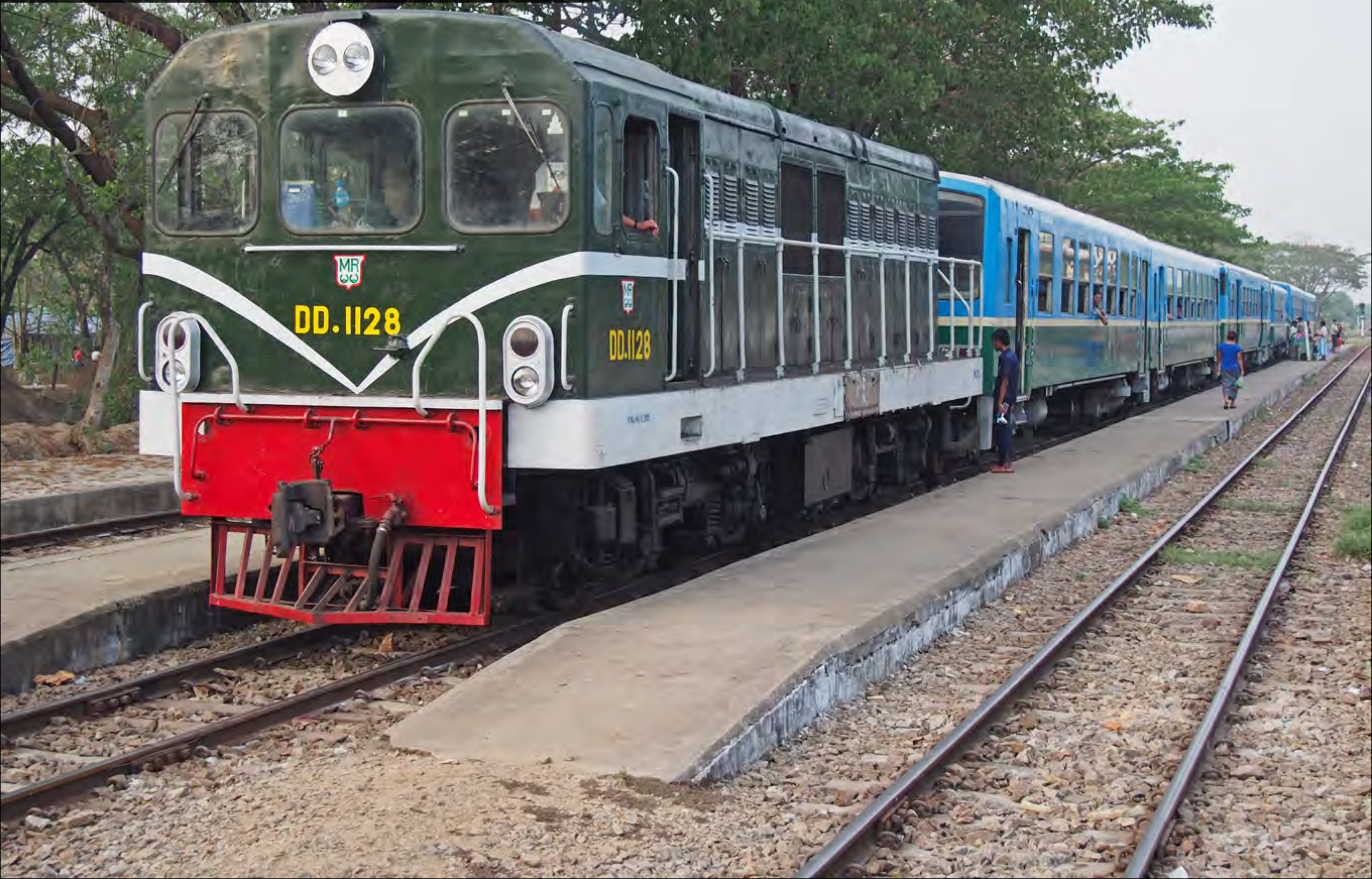
Sifang Locomotive and rolling stock company (China) built No. DD.1128 Bo-Bo diesel-electric locomotive equipped with a 12V180ZJ engine has just run round it's consist of former diesel railcars at Togyauungale whilst working a Yangon – Thilawa service on March 15th. David Pollock
