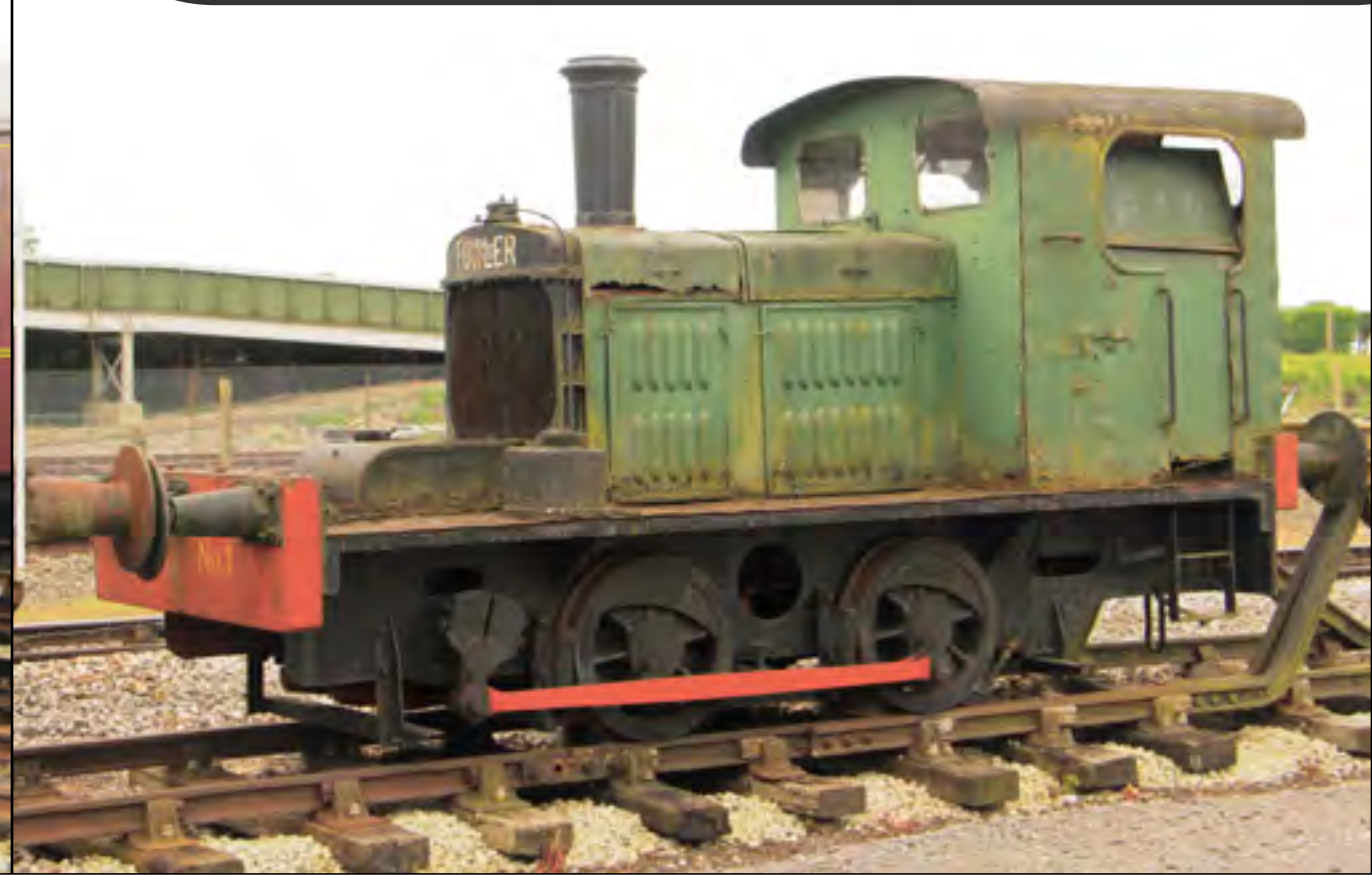
Fowler 0-4-0DM No. 20067 'Osram' awaits its turn for a full restoration at Quainton Road. Derek Elston
