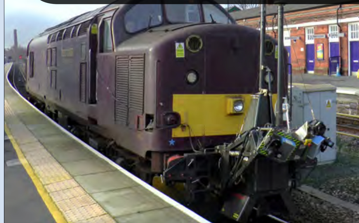
West Coast’s Class 37 706 calls at Stalybridge on January 11th with a Preston to Diggle loop test train. The contraption on the front is a Dutch invention and is the only one in the country, it sends out a 360 degrees laser and the loco can travel up to 70mph whilst getting a picture of what state the track is in. Brian Hewertson
