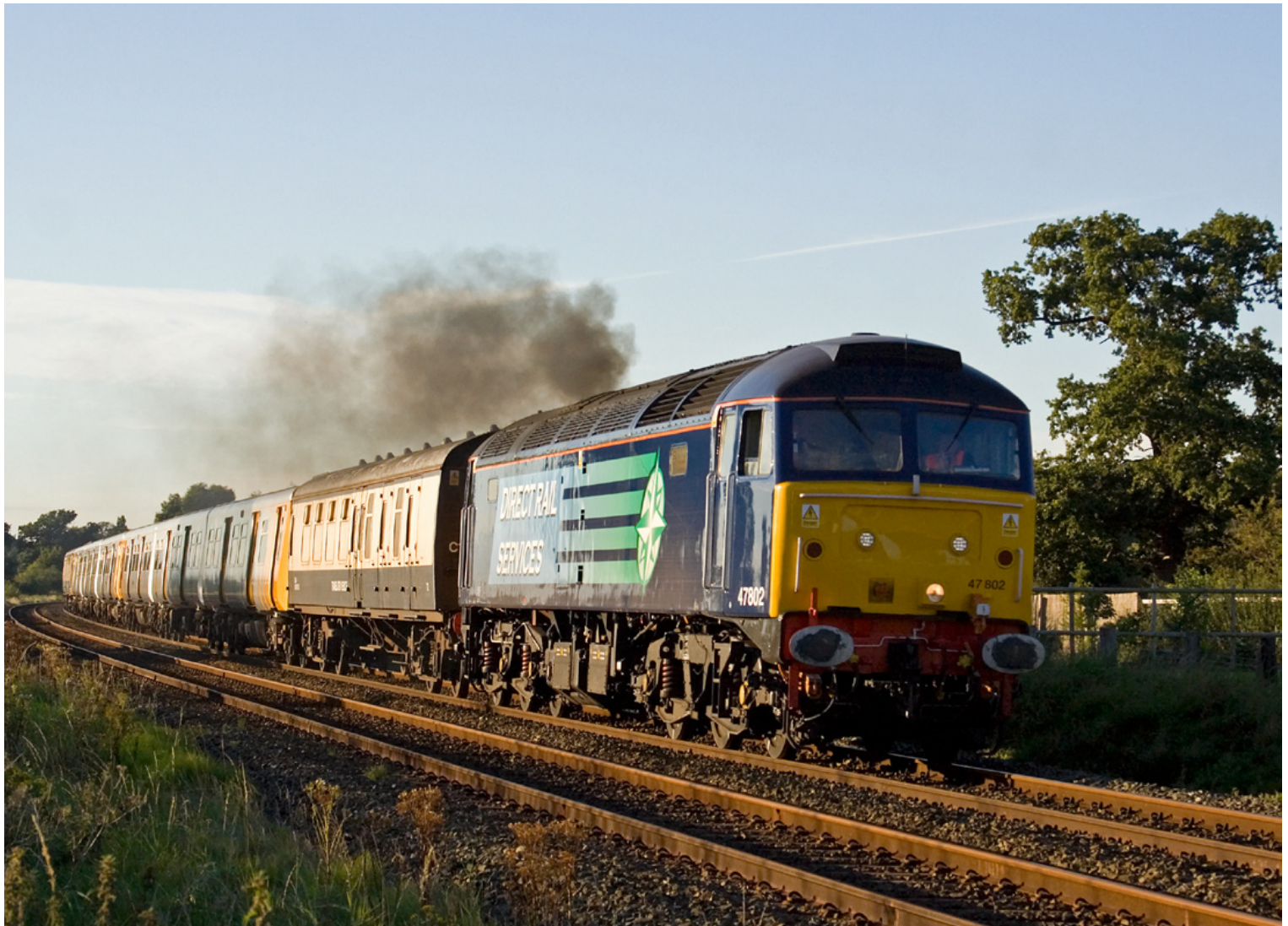
Above: 47802 passes Rowton on the 6th September with 7X47 Birkenhead North EMU Depot - Crewe CS unit move. Several 507/508s were being taken to various locations for tyre turning owing to excessive wheel wear. David Dawson
