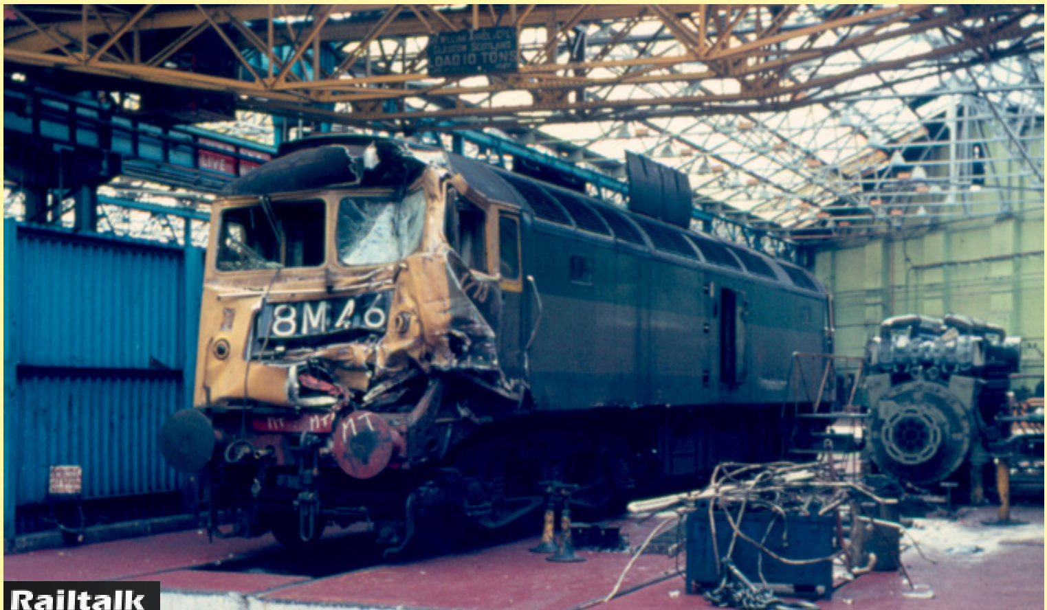
Below: Now Class 47's, but in 1970 still known as the Brush Type 4 D1713 inside Crewe Works having previously been involved in a collision. David Mead
