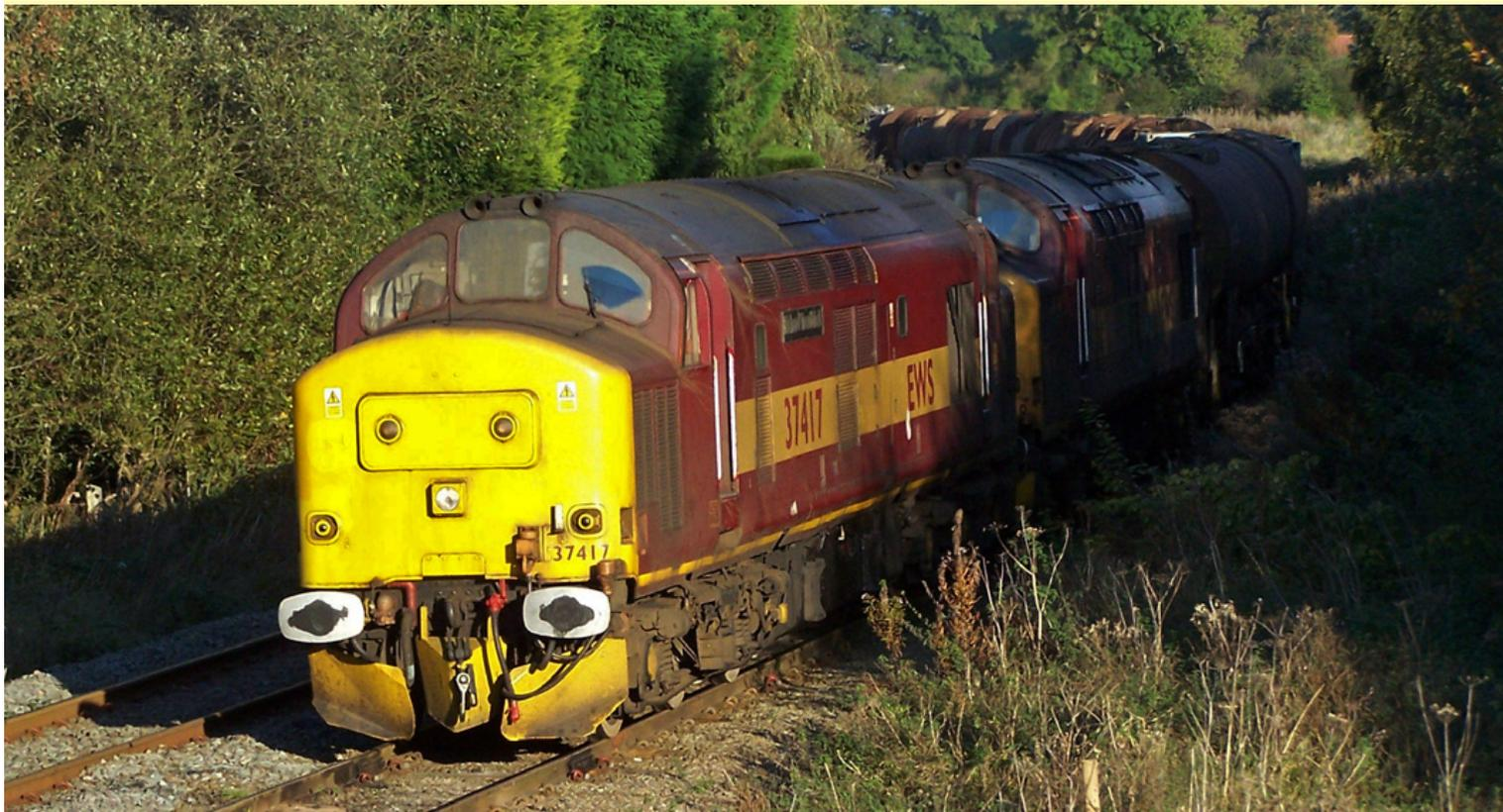
*Above: 37417 and 37410 at Hartford Junction on 19th October. This is a few miles south of Weaver Junction and is where the line from Northwich meets the WCML. The working is the 6F61 Folly Lane - Warrington which has started producing pairs of 37s due to the weight of the train making locos slip badly on the climb to Runcorn station. Mike Byrne*
