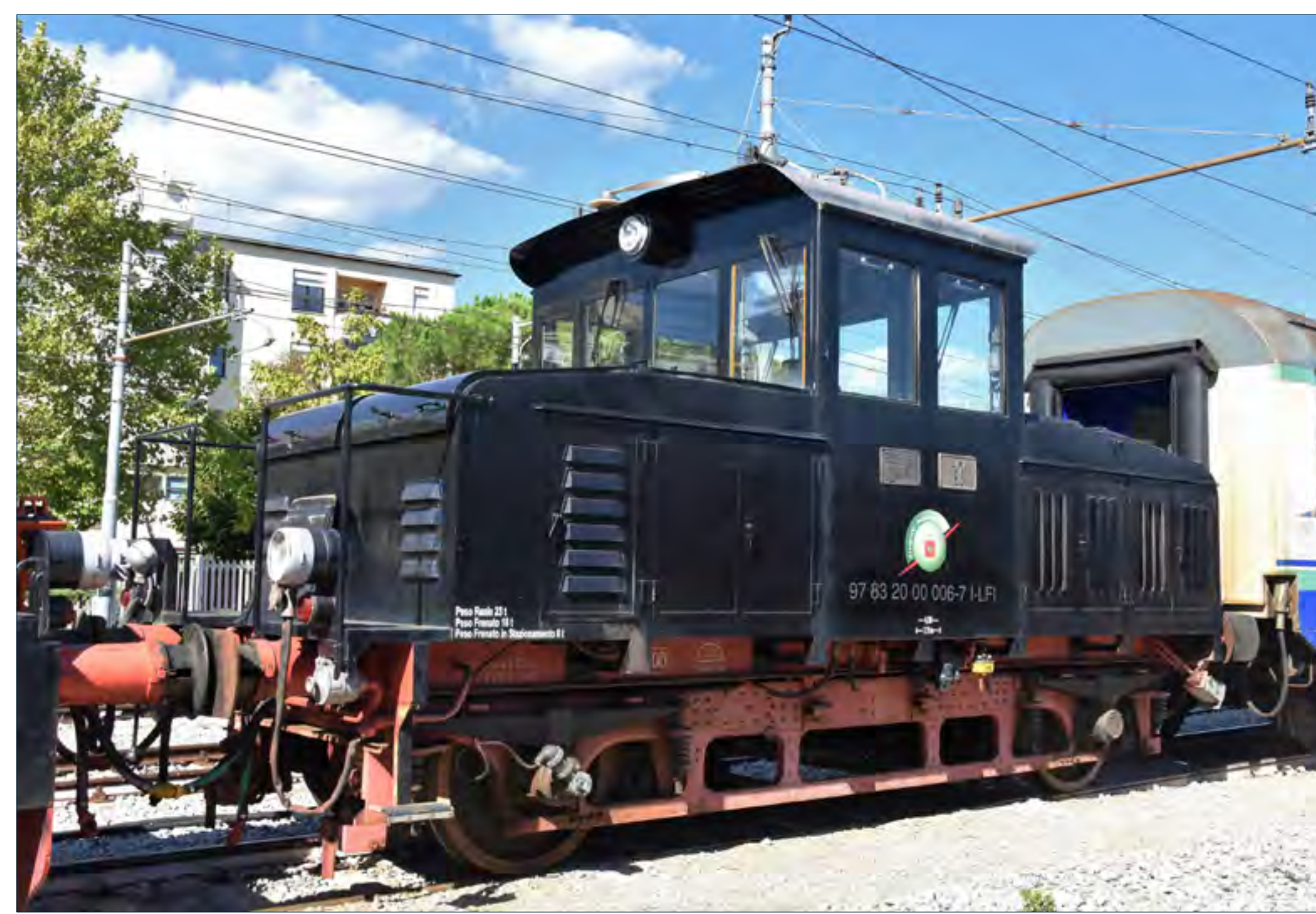
4w electric loco No. E6 built in 1950 stands in the yard at Arezzo Pesciola. John Sloane
