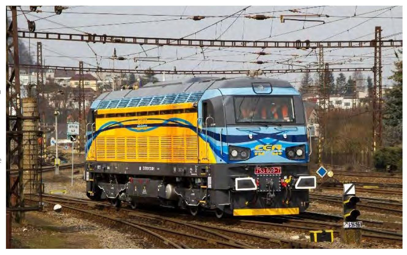
IDS Cargo's EffiLiner 3000 No. 385.001 speeds through Breclav with a loaded timber train. This loco was rebuilt by CZ Loko from SNCB Class 12 dual-voltage electric locomotive No. 1203. Class47
