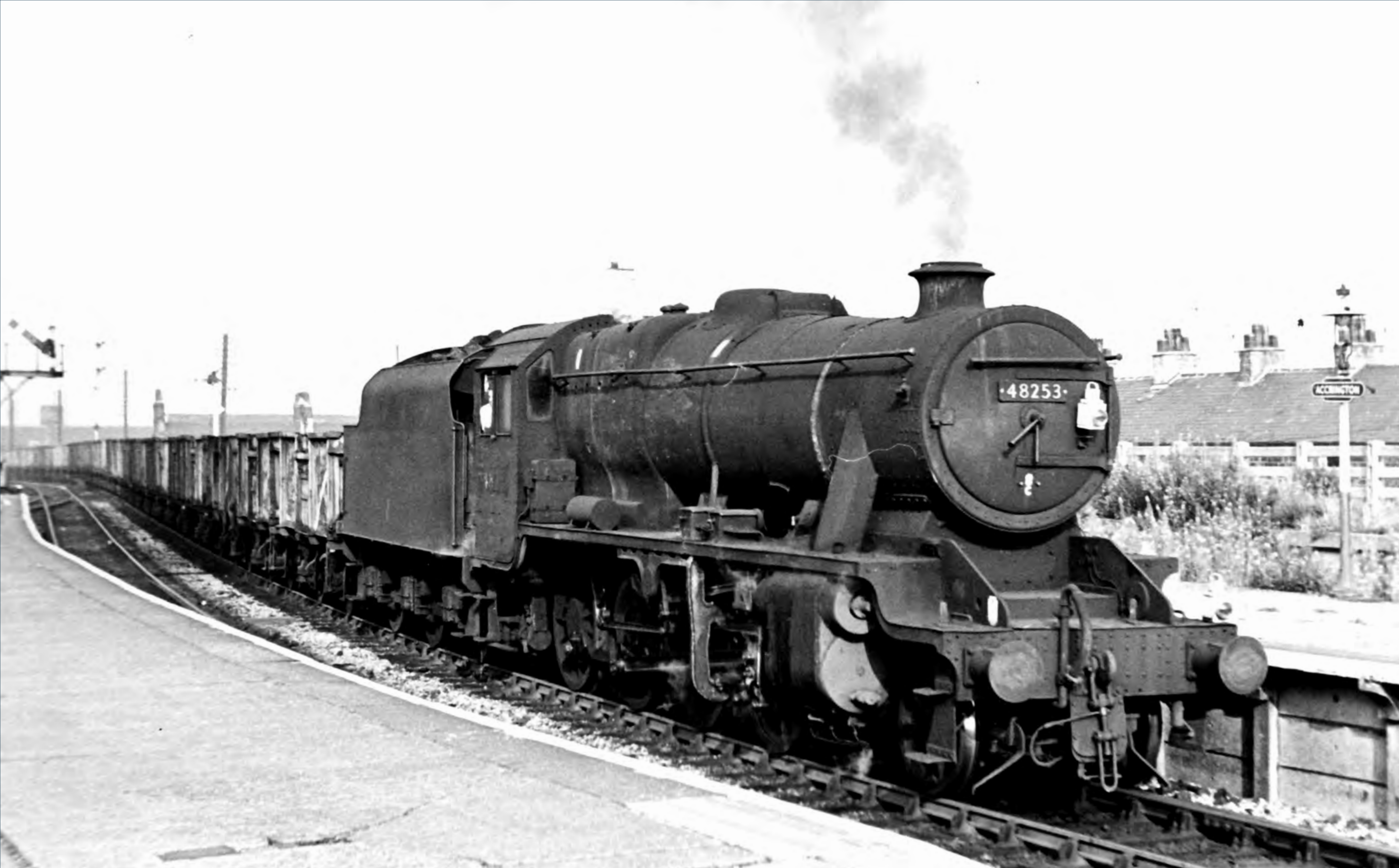
▶ Stanier LMS 8F Class No. 48253 passes through Accrington station with a long train of empty 16 ton coal wagons on July 8th 1967. Dave Felton
