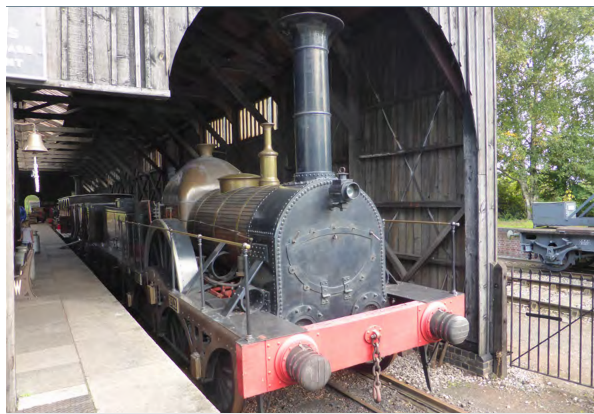
Broad gauge replica loco 'FireFly' was completed at Didcot by The Fire Fly Trust in 2005. The original was one of the first batch of a class of 61 locomotives designed by Daniel Gooch for passenger services on the Great Western Railway. It was built by Jones, Turner and Evans of Newton-le-Willows; introduced into service in 1840 and withdrawn in 1870.
