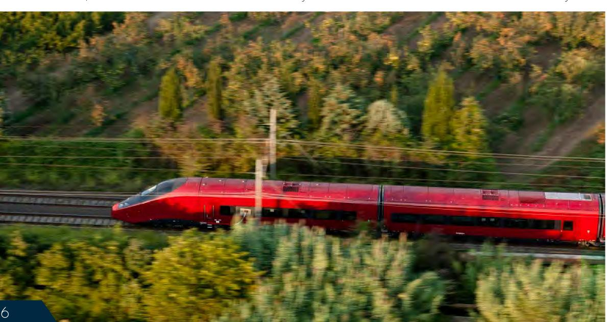
AGV is part of Alstom's Avelia range of high-speed trains. Able to run at commercial speeds of up to 360 km per hour, the AGV is equipped with a distributed traction system, tested at 574.8km/h in 2007 which set the last world speed record on rail. Featuring a futuristic and elegant aerodynamic nose, as well as the most modern technologies for very-high speed, the AGV won
