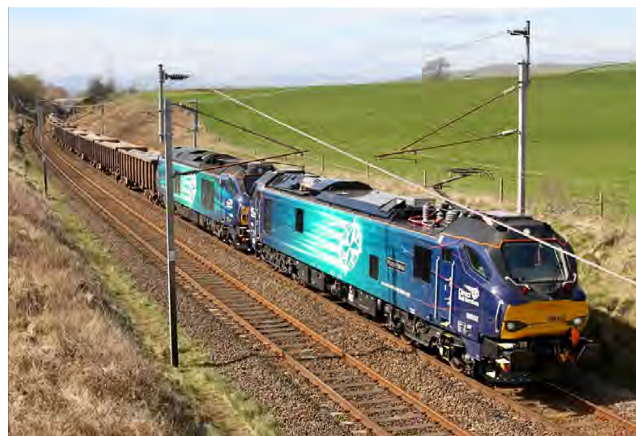
▶ Class 88 002 on its second day of loaded test running is seen heading north at Docker pulling 15 bogie wagons full of stone plus Class 68 025. Colin Kennington
