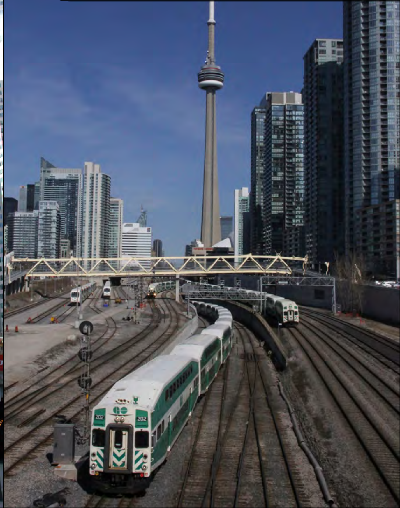
A Wabtec built MPExpress train departs from Union Station, Toronto on April 15th. With the CN Tower as a backdrop these trains run intensive services in the Greater Toronto area and feature DVT style cab trains (leading here) and 40,000 HP 93mph locomotives at the other end. Tim Ward
